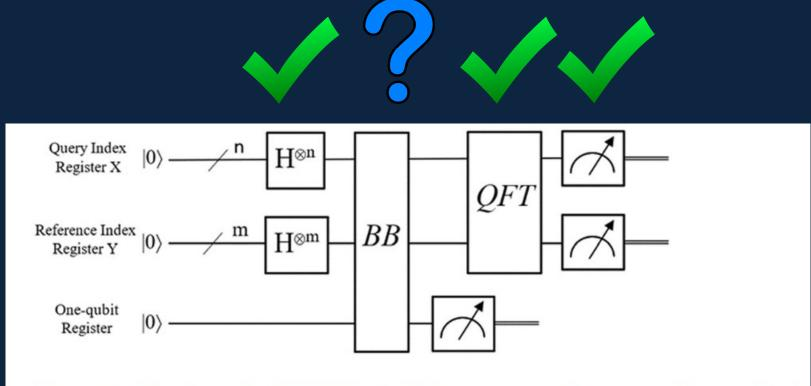
**Figure 1.** Circuit model of R. Schützhold's quantum pattern recognition method.
