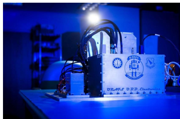
Air Force Research Laboratory's Optical Rubidium Atomic Frequency Standard, or ORAFS, is an advanced optical clock design built on existing vapor cell and laser technologies.
